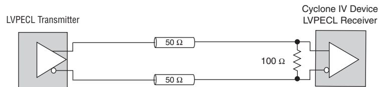
Figure 6-19. LVPECL DC-Coupled Termination (1)
