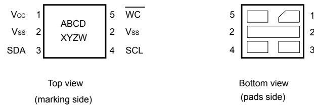
Figure 3. UFDFPN5 (DFN5) package connections
