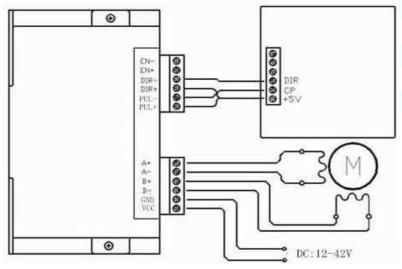
Logic control signals which have 5 V can be connected directly;
