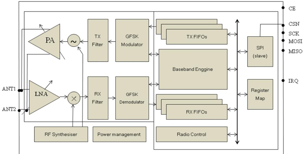
Figure1.1SE8R01 block diagram
