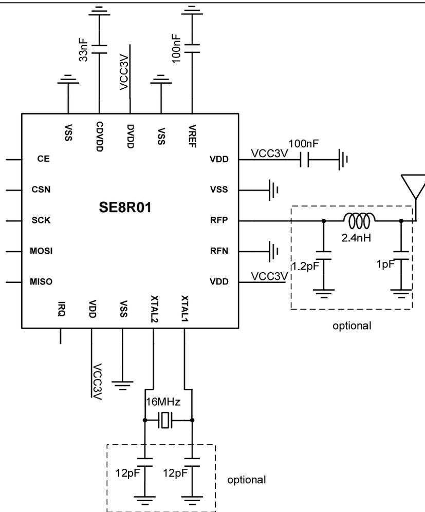
Figure 2.2 SE8R01 application circuit
