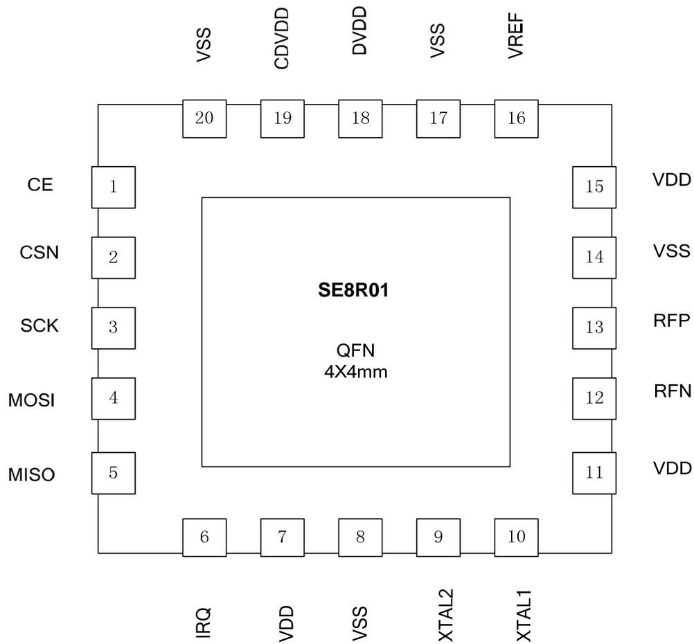
Figure2.1SE8R01 pin assignment (top view) for the QFN20 4x4 package
