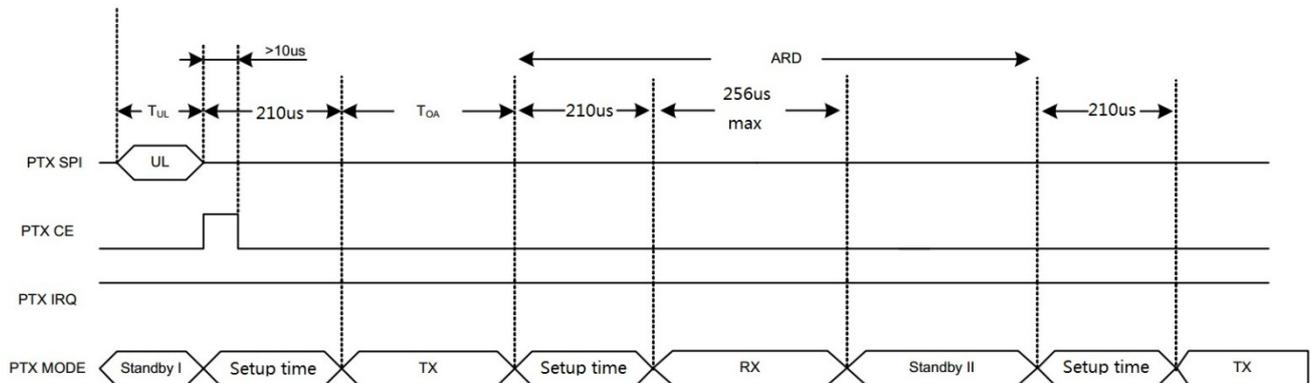
Figure 7.13 Timing of Protocol engine when the first ACK packet is lost (2 Mbps)
