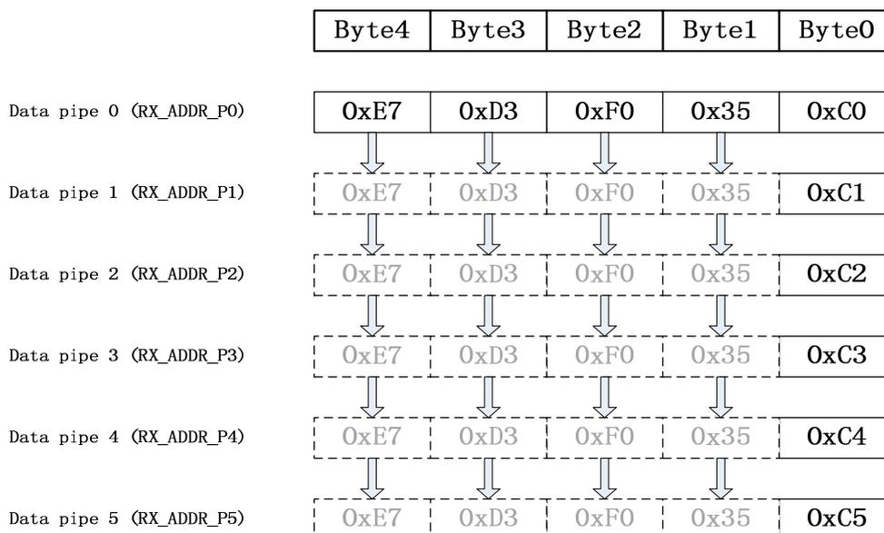
Figure 7.9 Addressing data pipes 0-5
