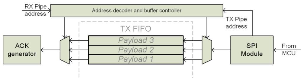
Figure 7.5 TX FIFO (PRX) with pending payloads
