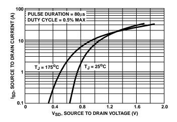
FIGURE 13. SOURCE TO DRAIN DIODE VOLTAGE
