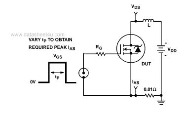
FIGURE 15. UNCLAMPED ENERGY TEST CIRCUIT
