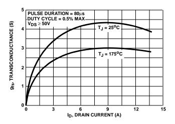
FIGURE 12. TRANSCONDUCTANCE vs DRAIN CURRENT
