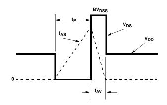
FIGURE 16. UNCLAMPED ENERGY WAVEFORMS
