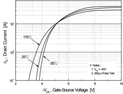
Figure 2. Transfer Characteristics
