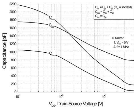
Figure 5. Capacitance Characteristics
