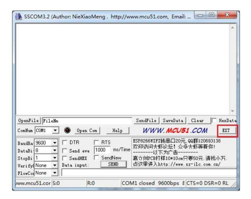
(3) Baud rate should be 9600. Tick HEX and HexData so that the command can be received by the Serial MP3 Player and you can see the feedback information (refer to the file **YX5300-24SS Datasheet V1.0.pdf**) in the blank of the window. Before sending commands, you should select the [ComNum] and click [Open Com].
