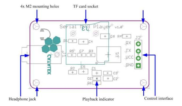
**Control interface:** It is UART TTL interface. A total of four pins (GND, VCC, TX, RX), GND to ground, VCC is the power supply, TX is the TX pin of the MP3 chip, RX is the RX pin of the MP3 chip.
