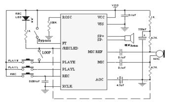
If you want change record duration, an external resistor is necessary to select the record duration and sampling frequency, which can range from 8 – 20 seconds (4-12kHz sampling frequency). The Voice Record Module of our provide default connect 100k resistor by short cap. So the default record duration is 10s.
