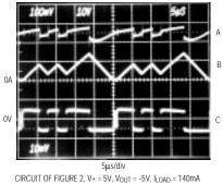
A: OUTPUT RIPPLE, 100mV/div B: INDUCTOR CURRENT, 500mA/div
