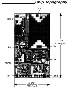
TRANSISTOR COUNT: 443 SUBSTRATE CONNECTED TO V+
