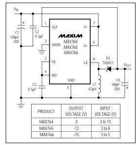
Figure 2. Fixed Output Voltage Operation
