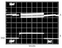
CIRCUIT OF FIGURE 2, V+ = 5V, V<sub>OUT</sub> = -5VA: V<sub>OUT</sub>, 50mV/div, AC-COUPLED B: ILOAD, OMA TO 100MA, 100MA/div
