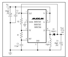
Figure 3. Adjustable Output Voltage Operation
