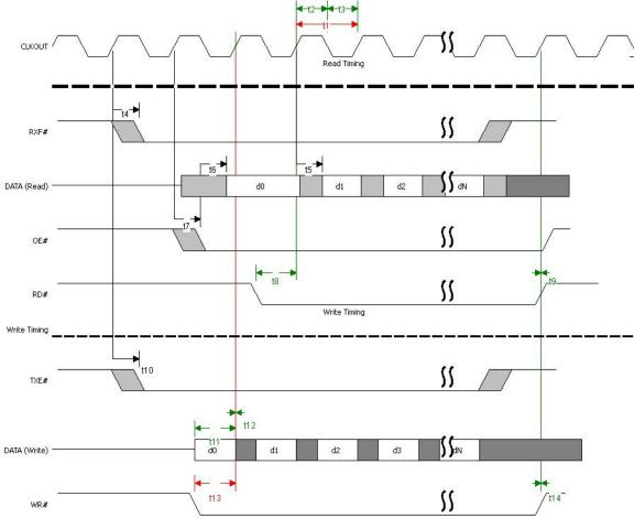
Figure 4.4 FT245 Synchronous FIFO Interface Signal Waveforms
