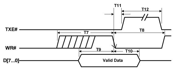
Figure 4.6 FT245 asynchronous FIFO Interface WRITE Signal Waveforms
