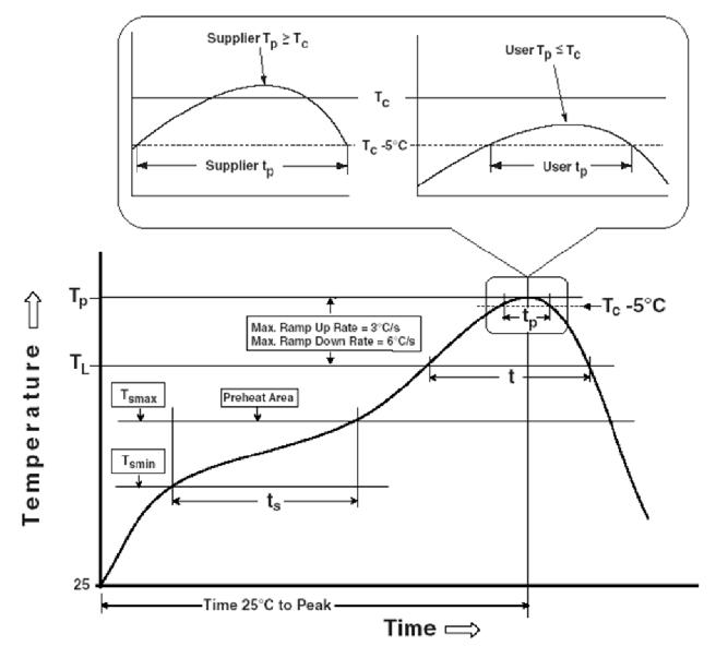
Figure 8.3 64 pin LQFP and QFN Reflow Solder Profile
