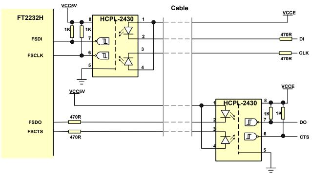
Figure 4.16 Fast Opto-Isolated Serial Interface Example
