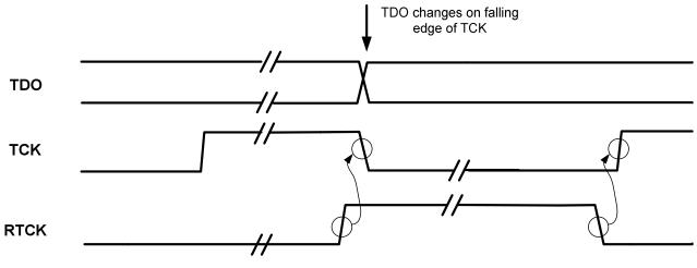
Figure 4.9: Adaptive Clocking waveform.
