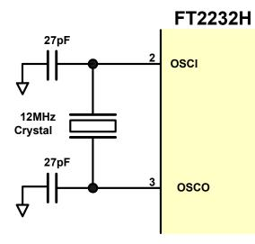
Figure 6.5 Recommended FT2232H Crystal Oscillator Configuration.
