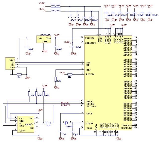
Figure 6.1 Bus Powered Configuration Example 1
