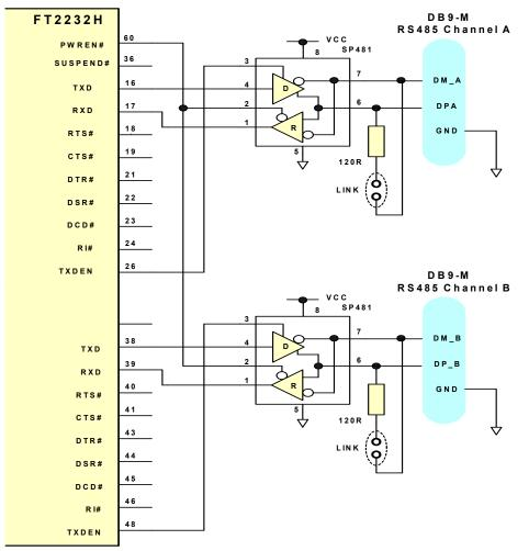
Figure 4.3 illustrates how the FT2232H can be configured as a dual RS485 interface.
