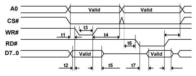
Figure 4.17 CPU-Style FIFO Interface Operation Signal Waveforms.
