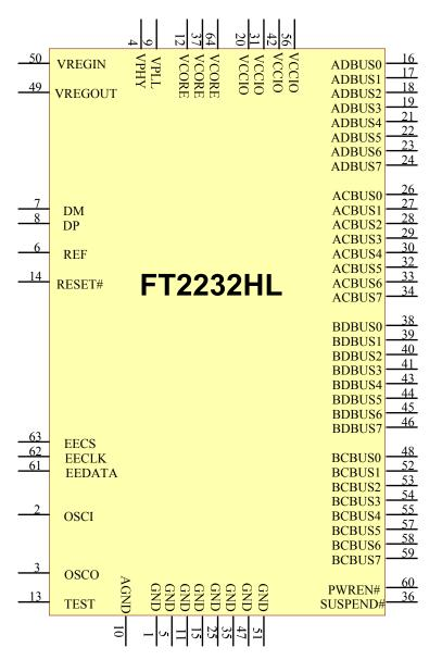
Figure 3.1 FT2232H Schematic Symbol
