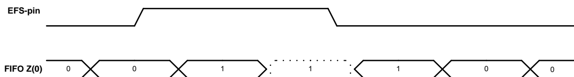
Figure 35: Timing diagram for external FIFO synchronization.
