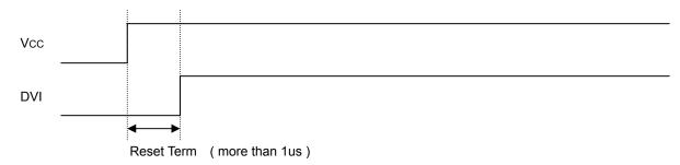
2) Timing chart2 for VCC and DVI supply. (If DVI rises within 1µs after VCC supply)
