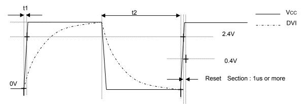
\* Please do the application design to secure Reset section 1us or more after the reclosing of the power supply.
