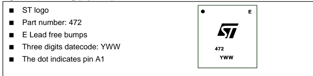
Figure 46. Flip-chip - 12 bumps
