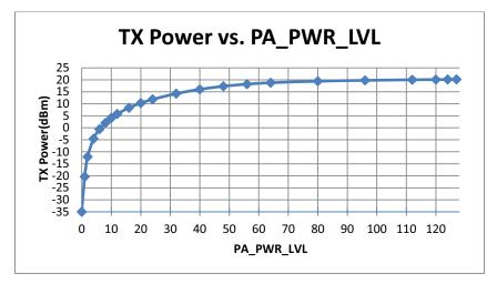
Figure 10. +20 dBm TX Power vs. PA\_PWR\_LVL
