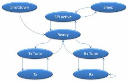
Figure 6. State Machine Diagram
