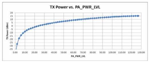
Figure 13. +13 dBm TX Power vs. PA\_PWR\_LVL
