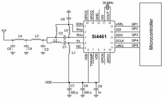
Figure 1. Si4461 Direct-Tie Application Example
