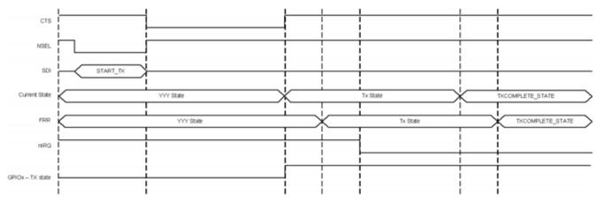
Figure 8. Start\_TX Commands and Timing
