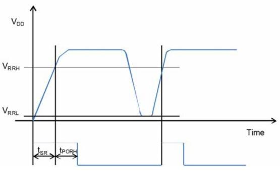
Figure 7. POR Timing Diagram
