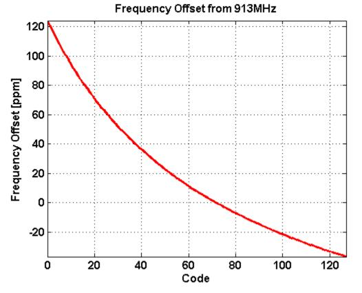
Figure 15. Capacitor Bank Frequency Offset Characteristics
