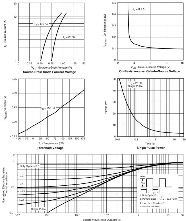
Normalized Thermal Transient Impedance, Junction-to-Ambient
