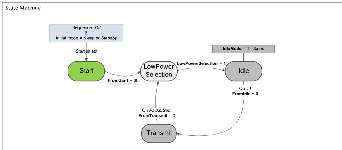
Figure 53. Beacon Mode State Machine
