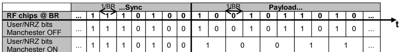
Figure 36. Manchester Encoding/Decoding
