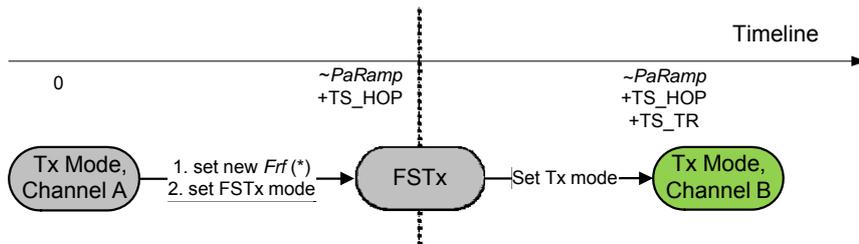
Figure 22. Transmitter Hopping
