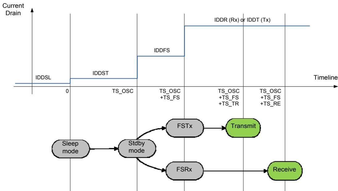
Figure 17. Startup Process
