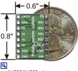
A4983/A4988 stepper motor driver carrier with dimensions.
