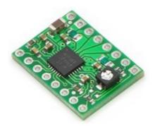
The A4988 stepper motor driver carrier is a breakout board for Allegro's easy-to-use A4988 microstepping bipolar stepper motor driver and is a drop-in replacement for the <u>A4983 stepper motor driver carrier</u>. The driver features adjustable current limiting, overcurrent protection, and five different microstep resolutions. It operates from 8 - 35 V and can deliver up to 2 A per coil.
