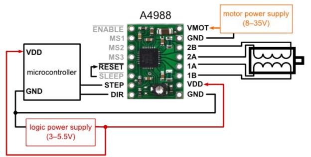
Minimal wiring diragram for connecting a microcontroller to an A4988 stepper motor driver carrier (full-step mode).
