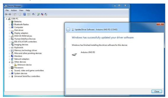
After driver is installed, go to "Device manager" again. Right click "Computer" —> "Properties"—> "Device manager", you can see UNO device as below figure shows, also the Comport info.
