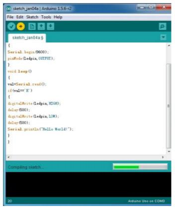
After uploading is done, open "serial monitor "; enter "R"; click "Send", the serial monitor will display "Hello World!" and the D13 LED will blink once.
