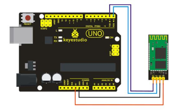
Now, let's move on to the program. I'll enter "r" and after Arduino receives my command "r", the pin13 LED on the main board will blink and serial monitor will print "keyes". The program is as follows:
