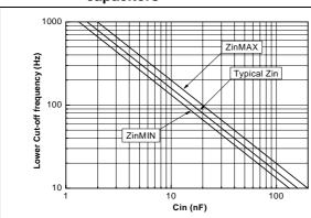
Figure 34. Lower cut-off frequency vs. output capacitors
