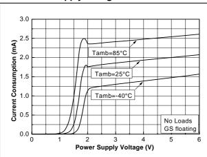
Figure 3. Current consumption vs. power supply voltage
