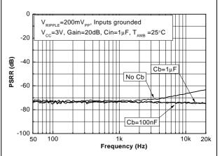
Figure 16. Single-ended output PSRR vs. frequency
