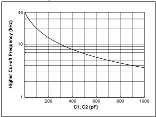
For example,  $F_{CH}$  is almost 20kHz with  $C_{1,2}$ =100pF.
