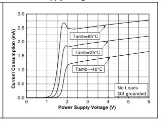
Figure 4. Current consumption vs. standby voltage
