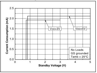
Figure 6. Standby threshold voltage vs. power supply voltage
