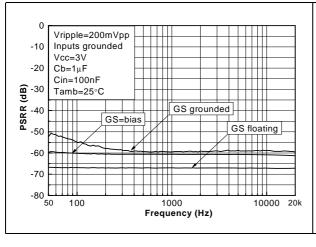
Figure 13. Differential output PSRR vs. frequency
