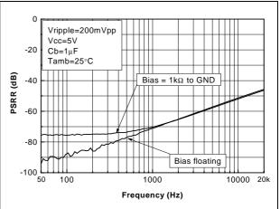
Figure 12. Differential output PSRR vs. frequency
