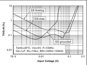
Figure 24. THD+N vs. input voltage
