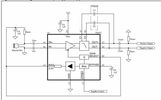
Figure 39. Single ended input typical application
