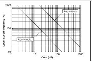
*Figure 33* and *Figure 34* give directly the lower cut-off frequency (with 3dB attenuation) versus the value of the input or output capacitors
